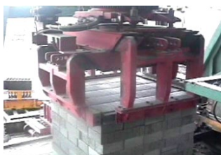
Cuber clamps blocks and stacks the on stock pallet in desired "cube".
