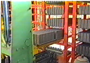
Blocks are unloaded from rack by Unloader
