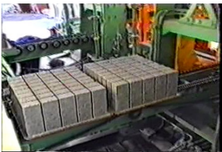
Unloaded locks are coming out on Unloader Chain Conveyor from Unloader
