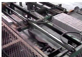
Pusher B arranges blocks under Cuber clamp
