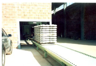
Cubed blocks on stock pallet comes out on Stock Pallet Roller Conveyor
