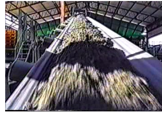
Aggregate transported toward Mixer by conveyor
