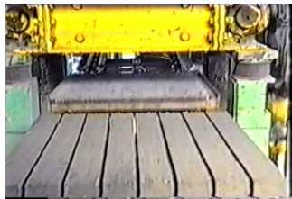
Green blocks are demoulded and come out onto Loader Chain Conveyor
